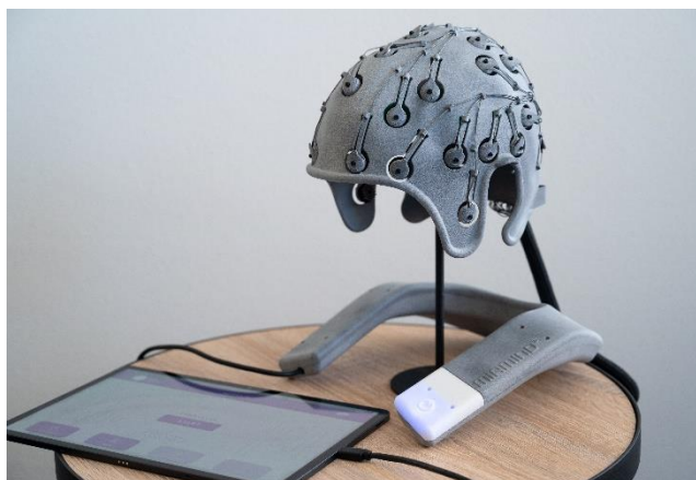
Custom-made MiamiMind® Neurostimulator. Portable tES & EEG device for repetitive diagnostic and treatment assessments at home
