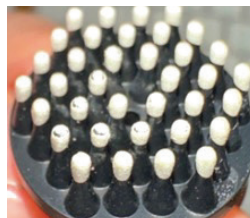
Example of damaged coating on the Miamind® electrode.
